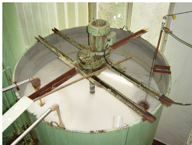
Fig. 10. Stirring of the filtrate during the industrial trial (KORTAN Company, Hradek nad Nisou).
